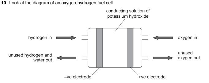
Potassium hydroxide solution contains potassium ions,  $K^{+}$ , and hydroxide ions,  $OH^{-}$ . Water,  $H_2O$ , is made in this type of fuel cell.
