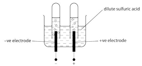
(a) Bubbles of gas are made at both electrodes.
