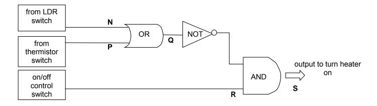
Truth tables can explain how an electronic system works.
