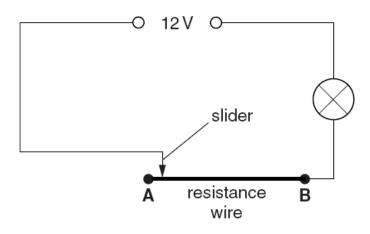
(i) Sally puts the slider at position A. The bulb lights up.
