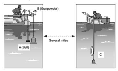
The bell (**A**) was struck and the gunpowder (**B**) ignited at the same time. The flash from the gunpowder and the sound from the bell were picked up several miles away (**C**).
