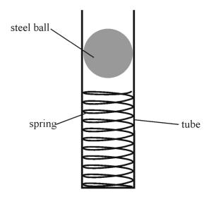
The spring is compressed, and the energy stored in the spring is used to fire the ball.
