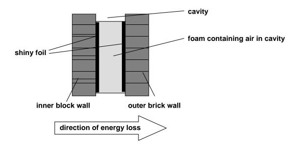
Describe how energy is lost through the wall from the inside to the outside **and** how the insulation reduces the different types of energy loss.
